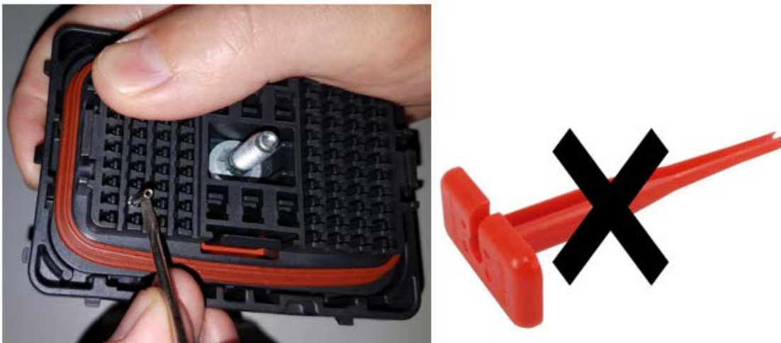
Figure 82 Removing a Contact from the Connector Housing Using a Small Screwdriver
