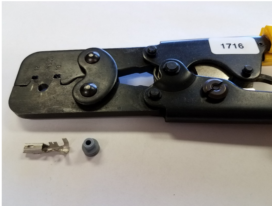
Figure 96 Yellow-Handle Waytek Crimper, 12 AWG Contact, and Gray Seal
