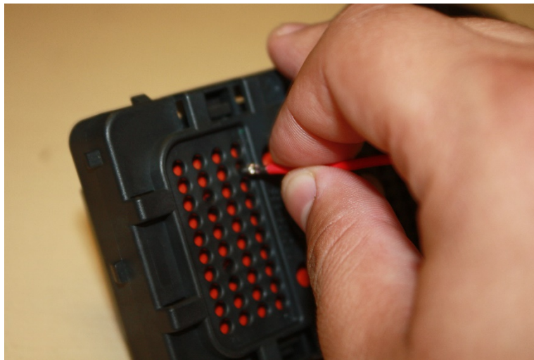
Adding a Wire/Contact to the Connector Housing
