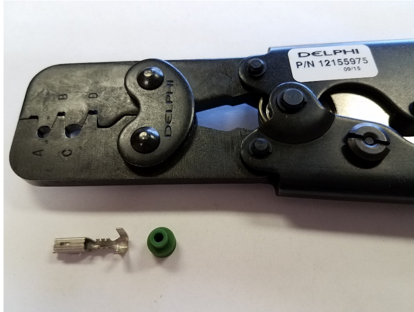
Figure 95 Black-Handle Delphi Crimper, 16-18 AWG Contact, and Green Seal
