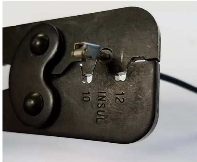
Figure 90 Crimping 12 AWG Seal with Slot INSUL Using Waytek Crimper
