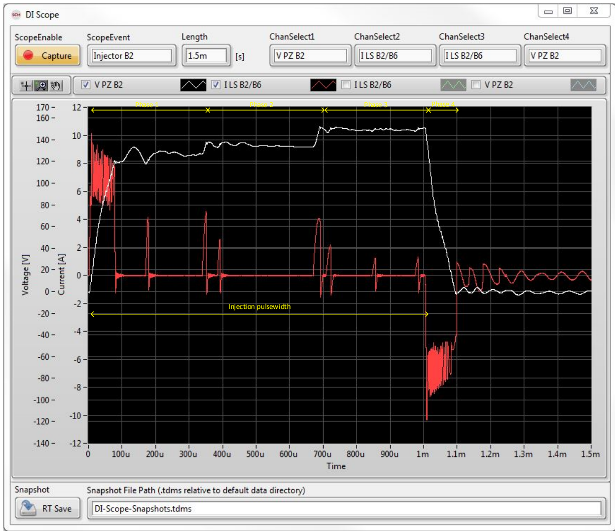
Figure 51 Piezo Injector Operation with Multiple Voltage Phases
