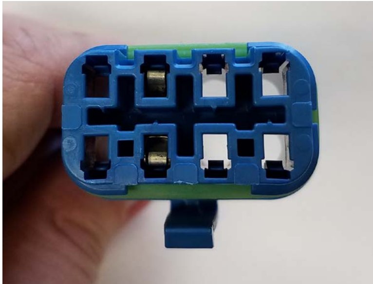
Figure 93 Proper Orientation of Fully Inserted Contacts (Notice the contacts are oriented in opposite directions when placed on opposite sides of the connector housing)
