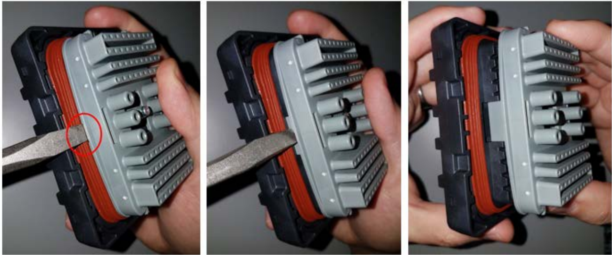
Figure 81 Removing the Contact Cover from the Connector Housing
