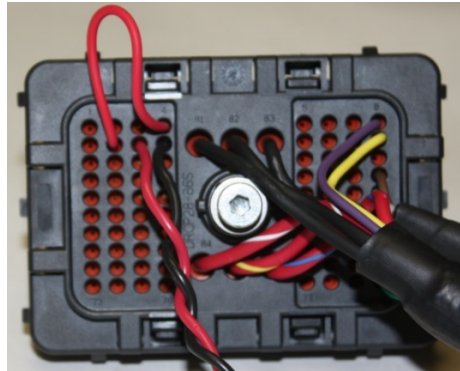
Figure 28. Example of a Jumper Wire Used for a Unipolar Piezo Injector
