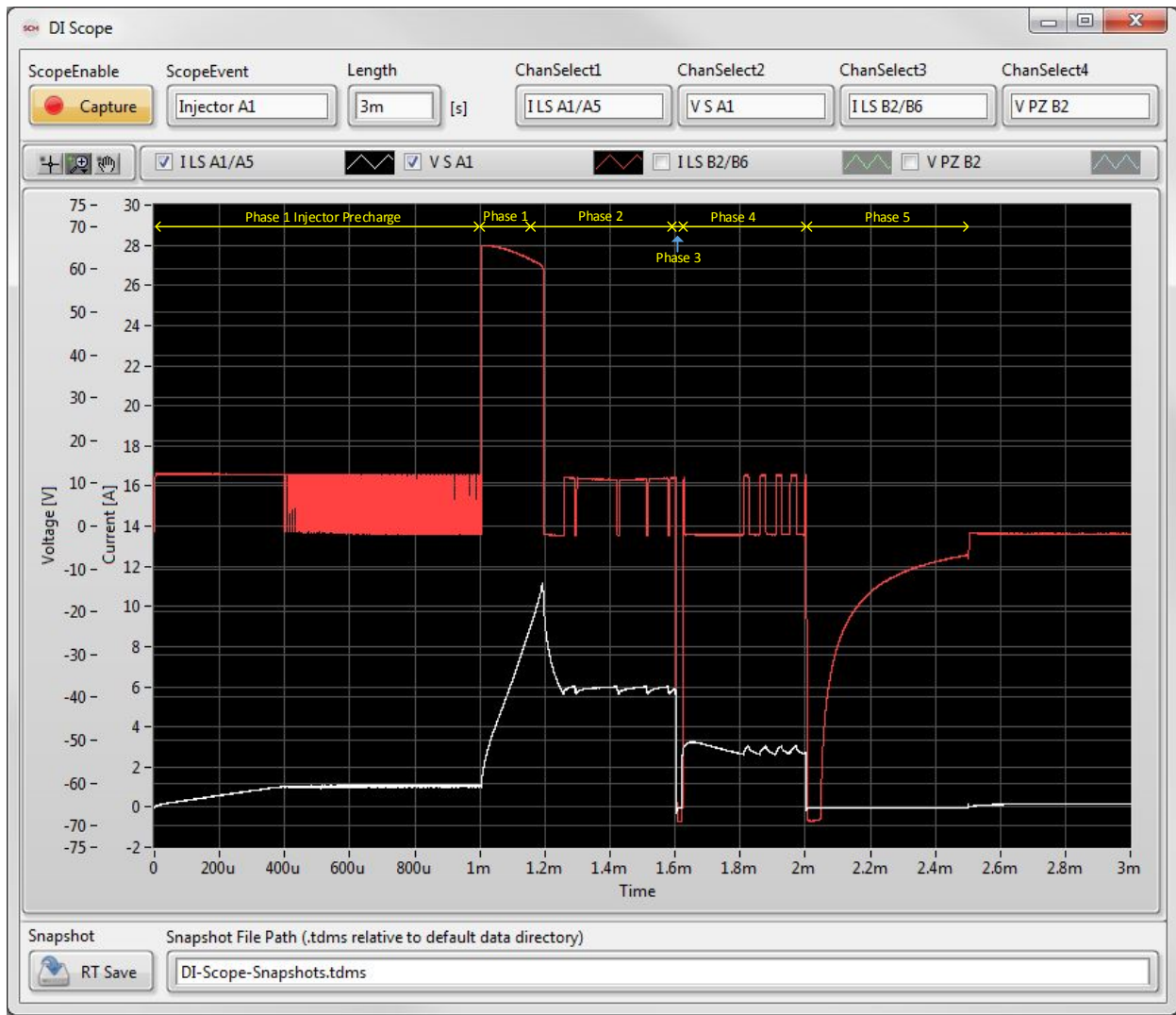
Figure 47 Plot of GDI Precharge Current and Voltage
