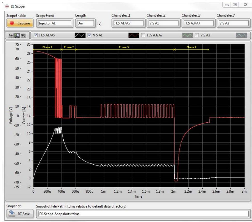
Figure 34. Basic GDI Operation with Backboost
