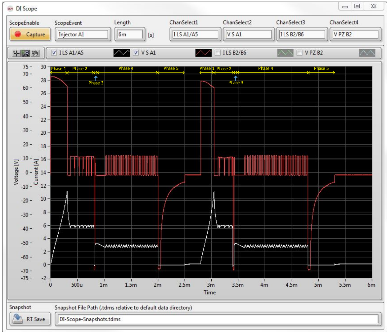
Figure 44. GDI Operation Using Multiple Phase Arrays
